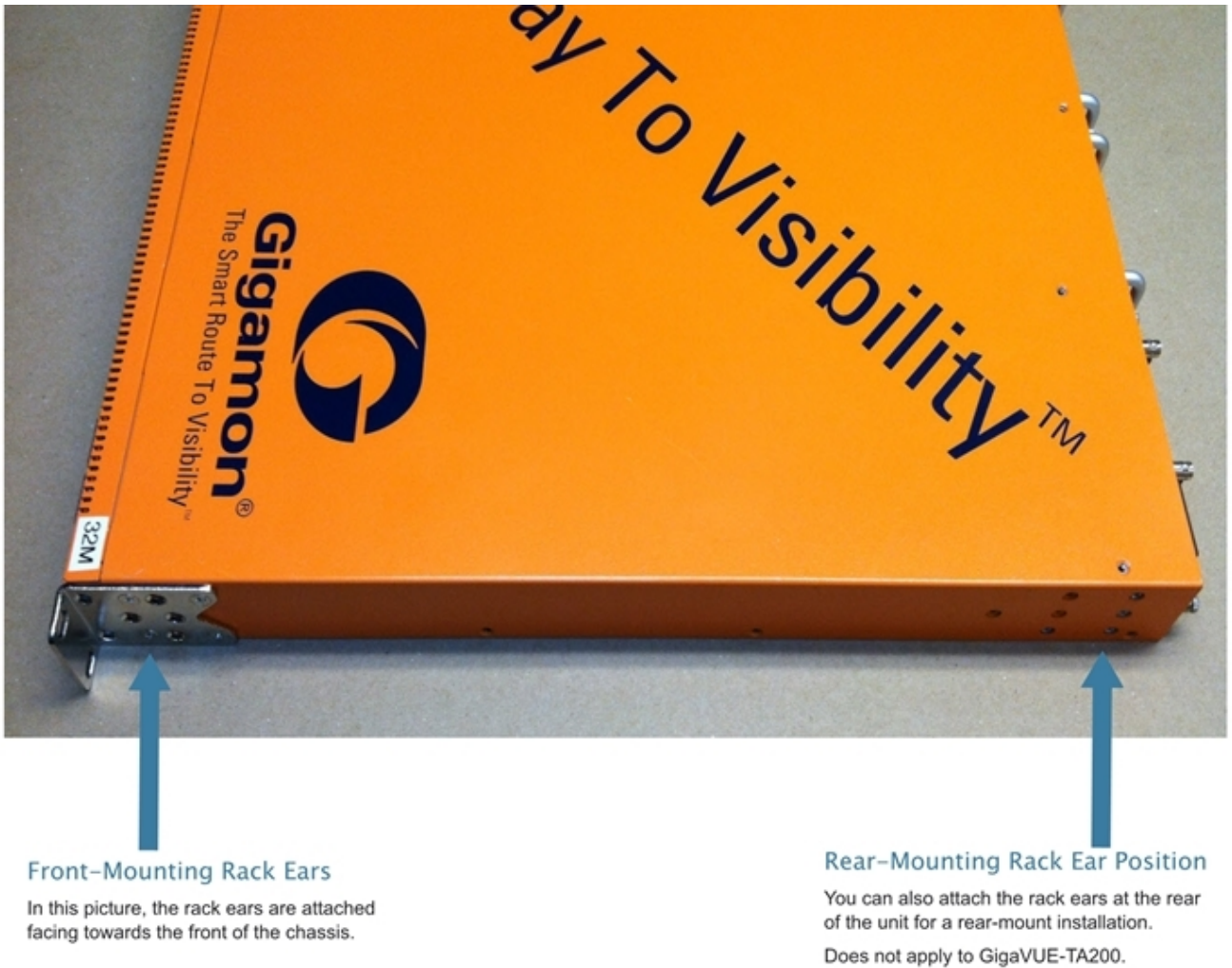
Figure 4 GigaVUE TA Series Traffic Aggregator Rack Ears in Front-Mount Position
