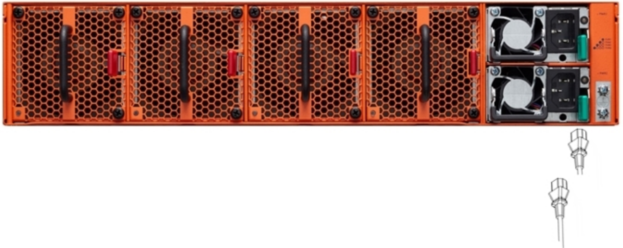
Figure 12 Connecting AC Power on a GigaVUE TA Series-TA200
